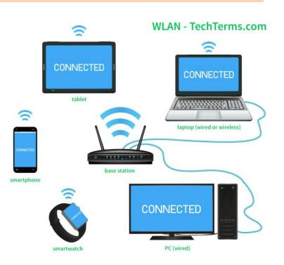
WLANs have data transfer speed ranging from 1 to 54 Mbps, with some manufacturers offering 108 Mbps solutions. The 802.11 n standards can be reaching 300 to 600 Mbps.
