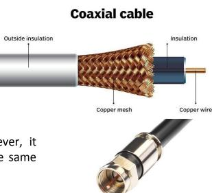
Due to the amount of shielding, coax cable is very resistant to cross talk and EMI (Electro Magnetic Interference)
